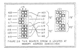
If 24-bit addressing is being used in the system, then J15 must also be set to correspond to address bits A16 through A23. See Figure 2.6.
