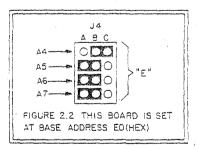
Secondly, the user should select the board I/O address. If the board is 8 bit addressed, then only jumper area J4 affects board address. The user may select address bits 4 through 7. See Figure 2.2. Finally, if the board is 16 bit I/O addressed, then jumper area J19 affects the upper 8 bits of board address, A8 through A15. See Figure 2.3.
