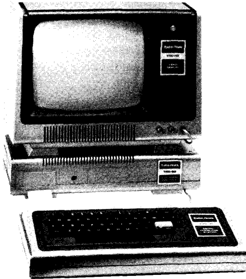
Figure 7. Set up your TRS-80/Expansion Interface/Video Display system this way.
