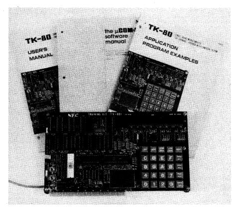
Single step operation Trace system status including all CPU registers and flags Modify CPU registers and flags Store and load memory to and from external audio cassette tape.
