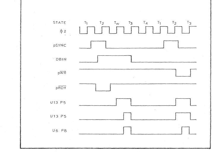
As an example, consider the sequence of events during an address breakpoint on input port number FF while running the FF PORT TEST PROGRAM.
